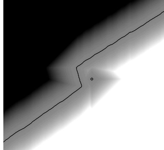
Fig. 7: The pre-calculated distance map. White and black values represent large distances (black when inside walls).
