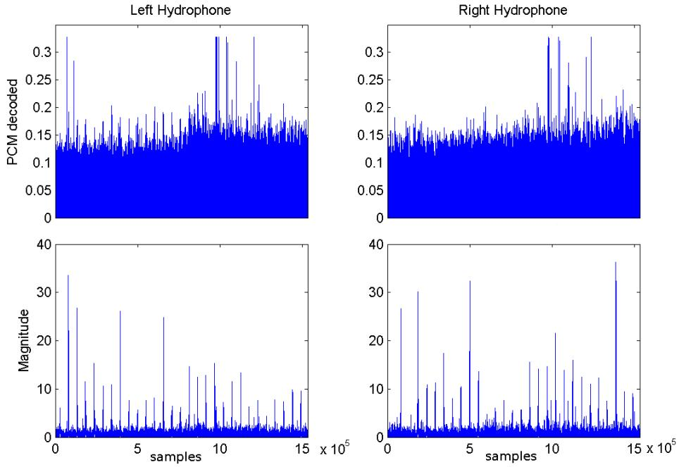
Fig. 9: Frequency analysis of the stereo hydrophone signal in presence of noise. The top plots show the raw signal, the bottom plots show the signal magnitude at the target frequency as estimated by the sliding Goertzel algorithm.
