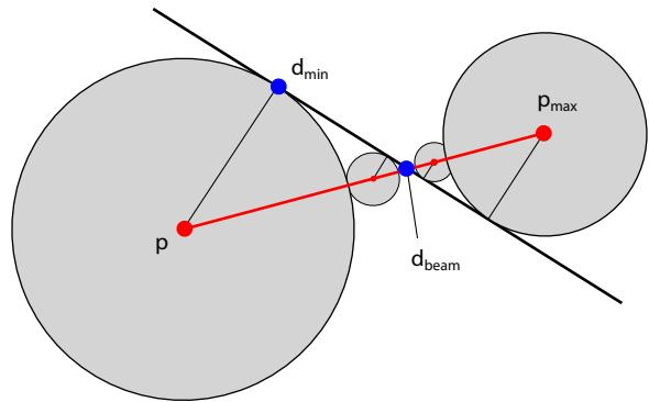
Fig. 8: Rather than considering the nearest neighbour  $d_{min}$  of a wall feature  $p$ , the nearest neighbour along the sonar beam (red line),  $d_{beam}$  is estimated. This is solved iteratively starting at point  $p$  and the point  $p_{max}$ , which is defined by the maximum sonar range along the beam. Using the distance map and a combination of bisection search and ray marching,  $d_{beam}$  can be efficiently estimated.
