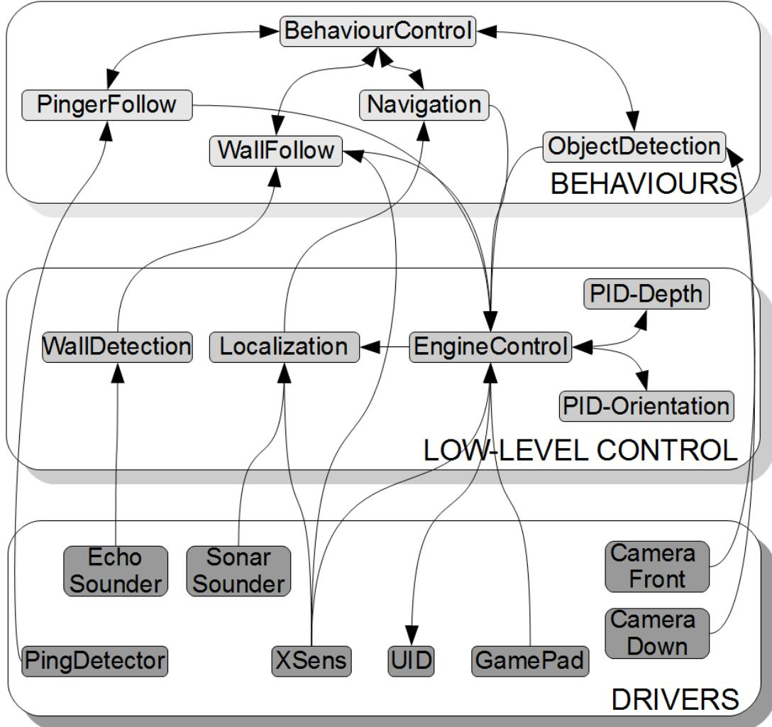
Fig. 4: The three-level software overview for HANSE. Each part represents a ROS Node. Arrows represent a communication between nodes through topics.
