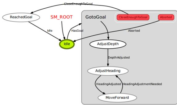
Fig. 5: SMACH state machine for the navigation behaviour.
