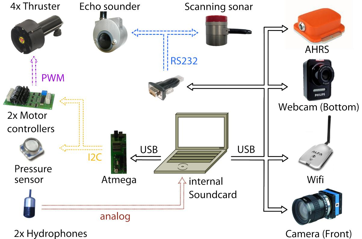
Fig. 2: Hardware overview of the HANSE AUV.
