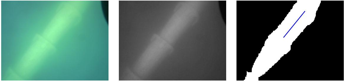
Fig. 3: Object detection using segmentation. Left: RGB image. Center: segmentation channel (red). Right: Otsu thresholding. The blue line indicates the position and direction of a yellow pipeline.
