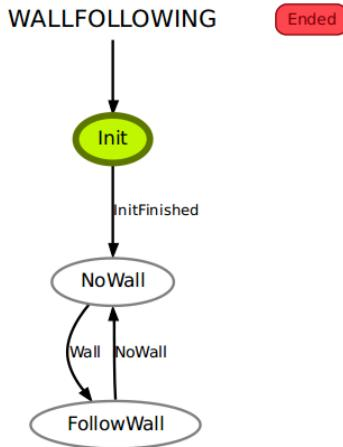
Fig. 6: SMACH state machine for the wall following behaviour.
